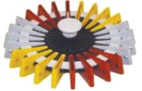
24 Blood ID Rotor Specific program for blood type card Step 1: 2min 55x g 800r/min Step 2: 3min 200x g 1500r/min
